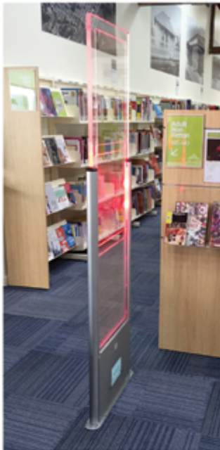
A subtle yet still visible LED alarm signal is triggered by items that have not been checked out.
